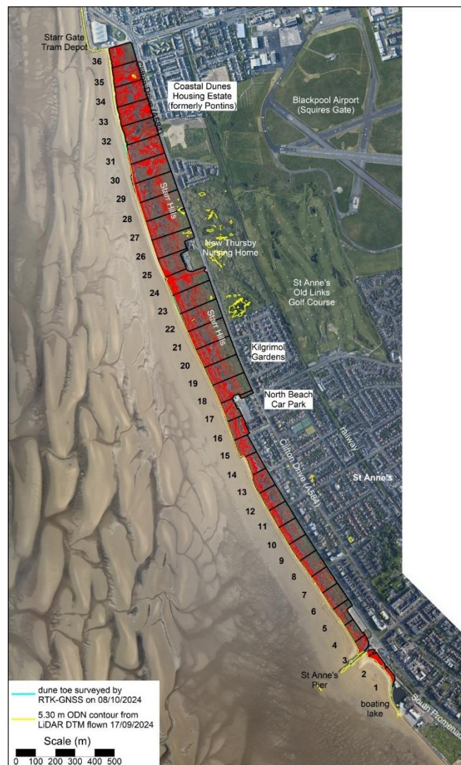
Figure 30. Extent of bare sand (red) in the dunes at St Anne's North Beach superimposed on aerial photography flown 11/05/2024. The positions of 36 defined dune cells (100 wide) are also shown. Photography source: Channel Coastal Observatory
