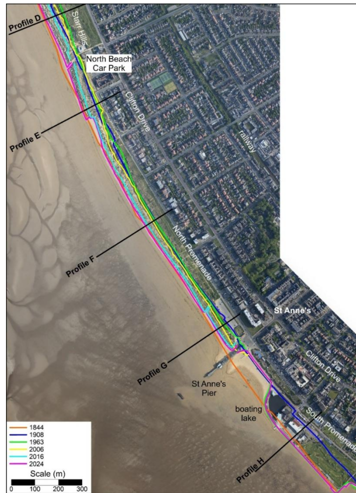
Figure 23. Aerial photography of the Lytham St Anne's area flown 11/05/2024, overlain with historical positions of the dune toe from OS maps (surveyed 1844, 1908 and 1963), aerial photography (2006, 2016 and 2024) and RTK-GNSS survey (07/03/2016 and 08/10/2024). Source: Channel Coastal Observatory
